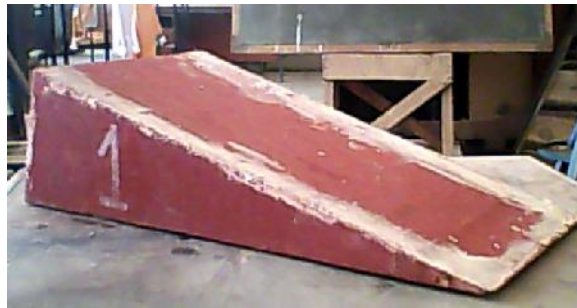
Plate II: Model 1 of apex angle 80^\circ , upstream angle and slope, 85^\circ and 0:1, downstream angle and slope, 15^\circ and 4:1 respectively.
