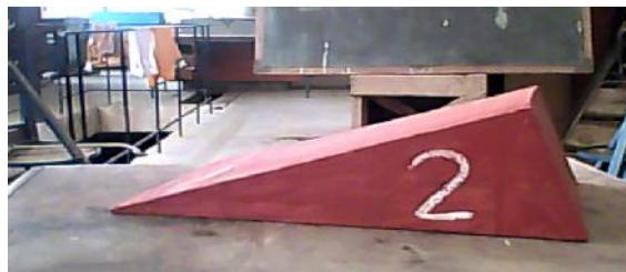
Plate III: Model 2 of apex angle 90^\circ , upstream angle and slope, 70^\circ and 0:3, downstream angle and slope, 20^\circ and 3:1 respectively.
