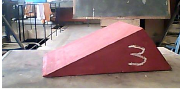
Plate IV: Model 3 of apex angle 100^\circ , upstream angle and slope, 55^\circ and 0:7, downstream angle and slope, 25^\circ and 2:1 respectively.
