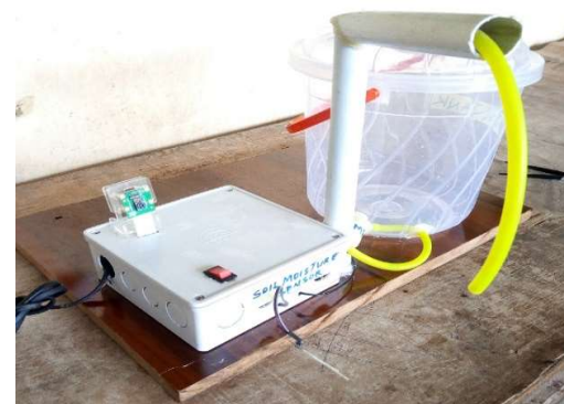
Figure 9: The Developed IoT Based Irrigation Control System.
